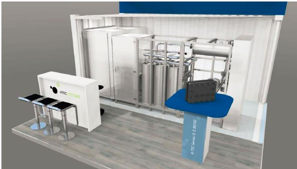
The H-TEC SYSTEMS electrolyzers convert electricity into hydrogen extremely efficiently at an efficiency rate of approx. 75 percent.
